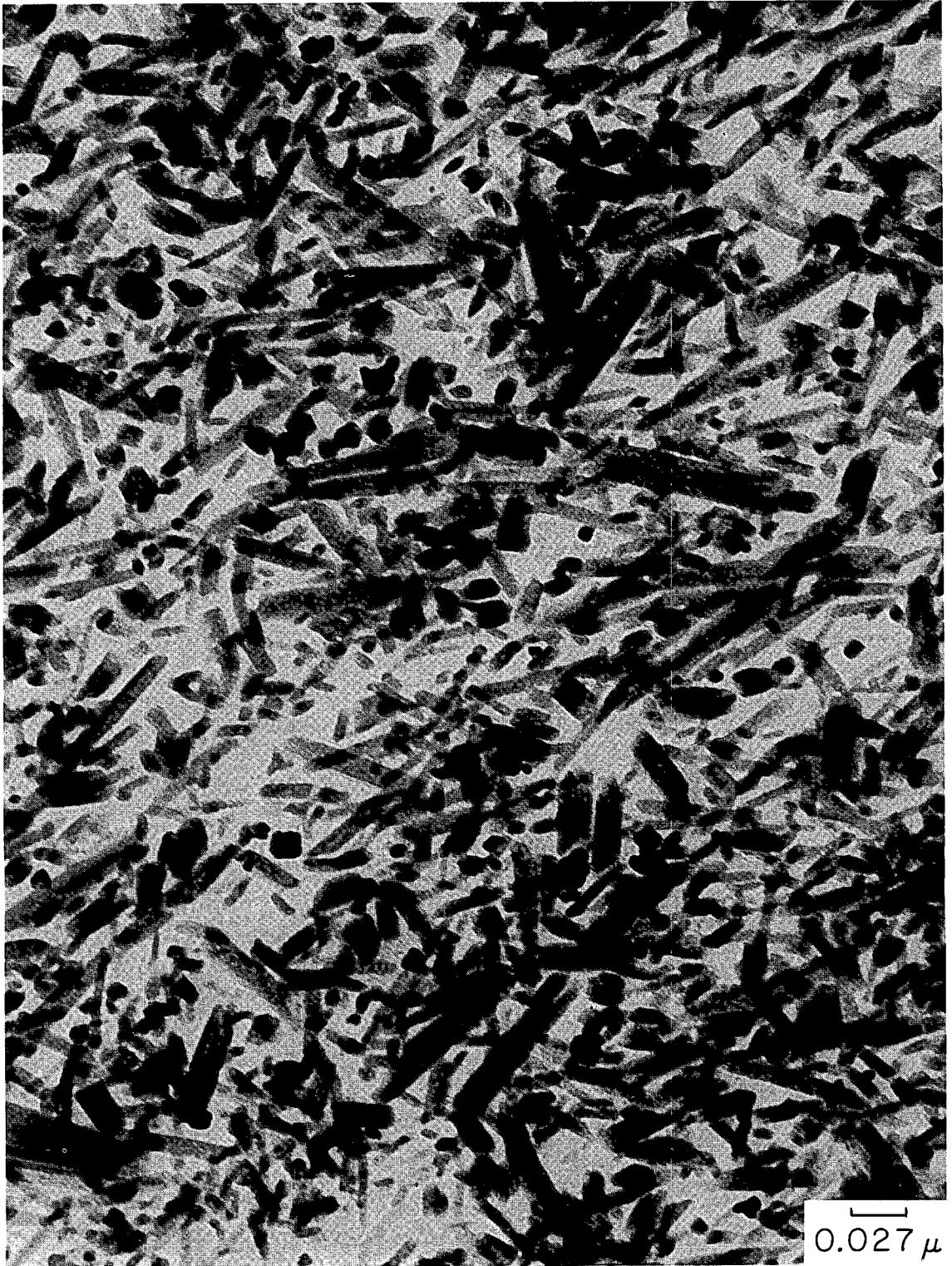
Fig. 7. Microtomed Cross Sections of Pr Sol-Gel Beads.
