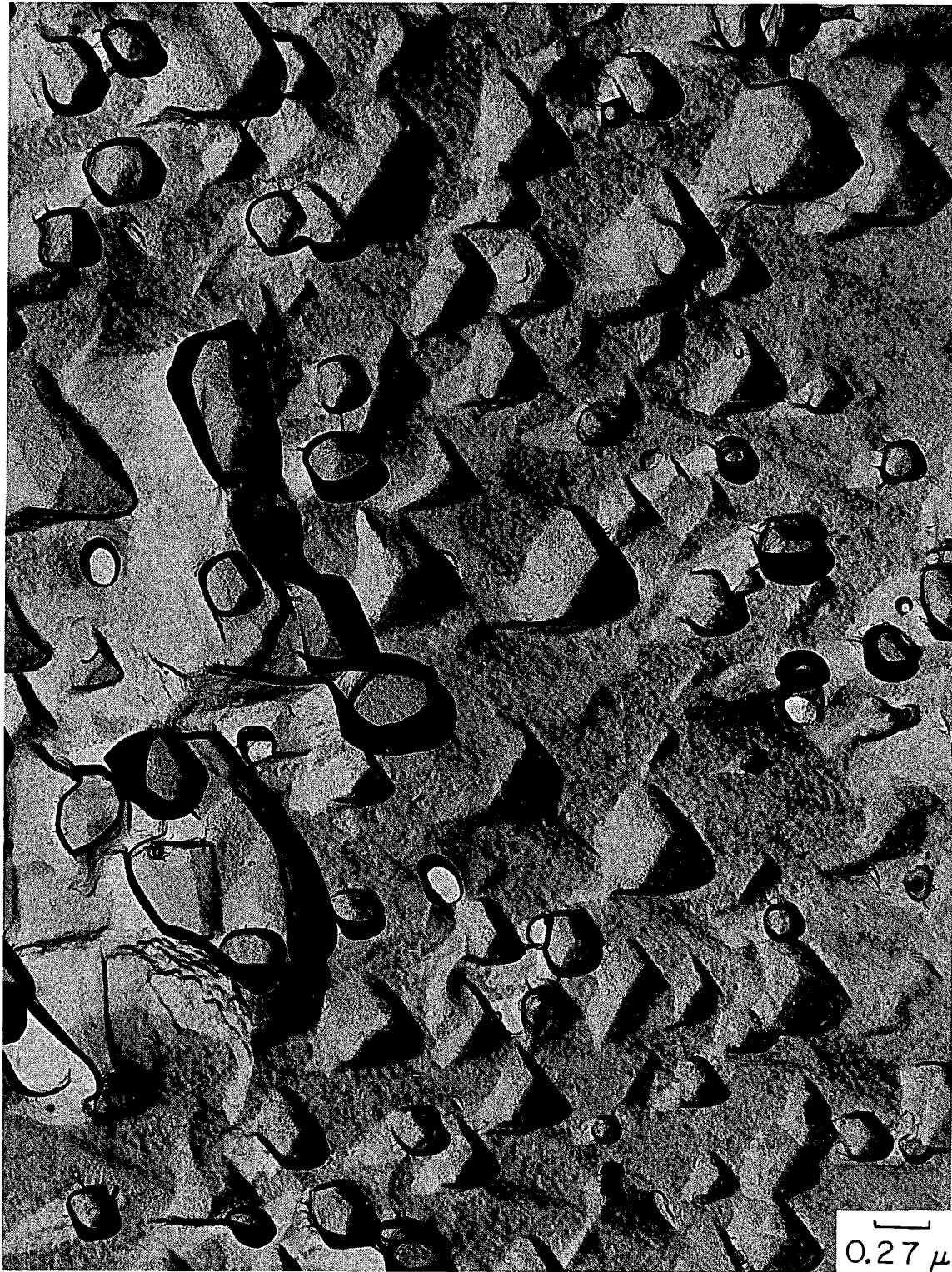
Fig. 20. Polished and Etched Cross Section of \text{Eu}_2\text{O}_3 Microspheres Calcined at 1400\text{-}1450^\circ\text{C} for 3 hr Showing the End Faces of Crystals.
