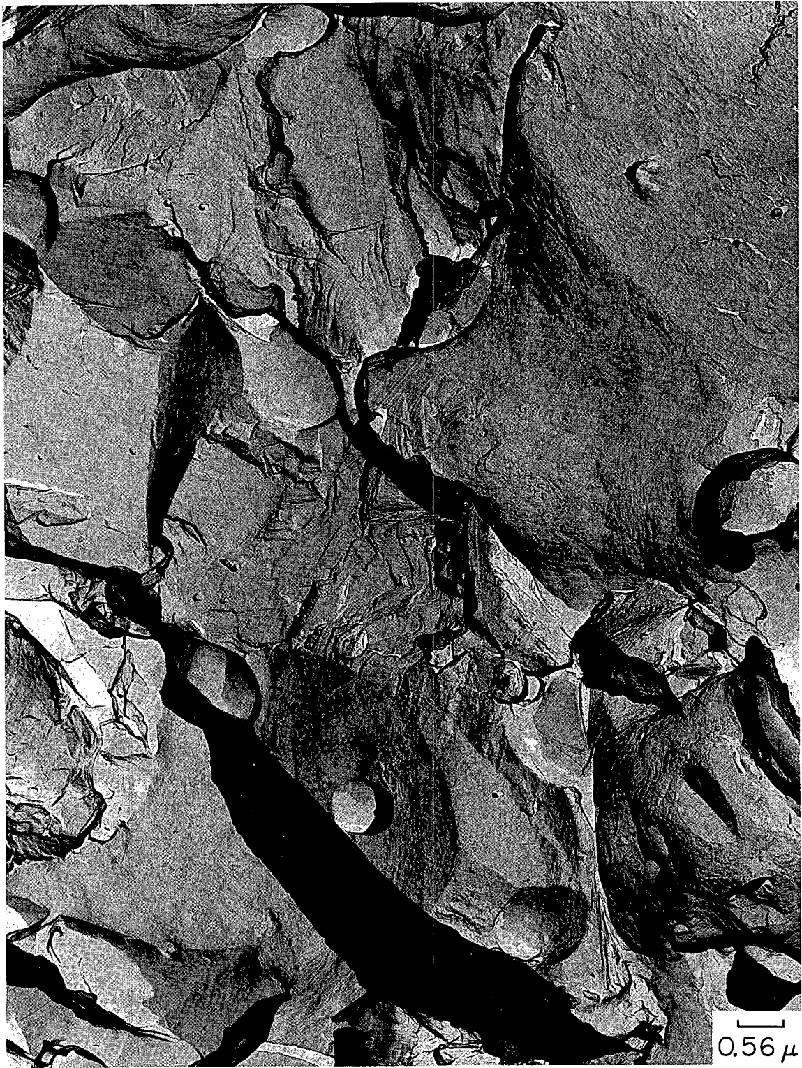
Fig. 22. Fractured Surface of \text{Eu}_2\text{O}_3 Microsphere Calcined at 1400-1450°C for 3 hr.
