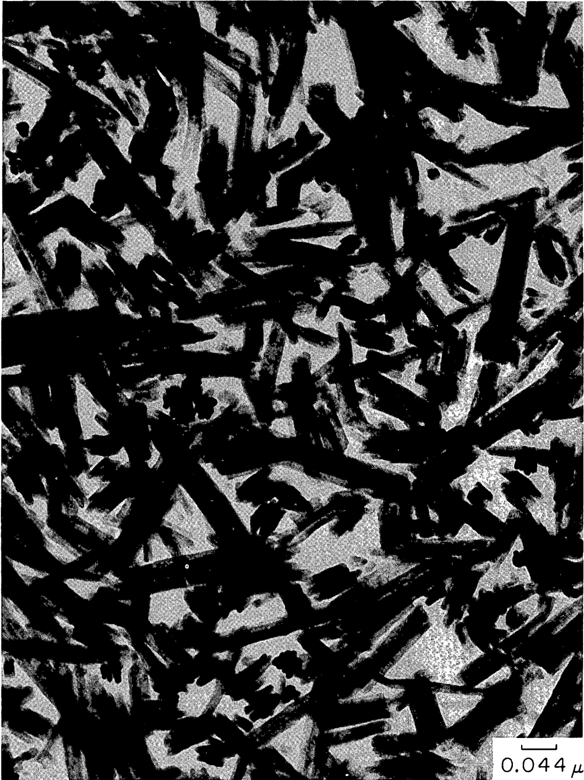
Fig. 8. Microtomed Cross Sections of Eu Sol-Gel Beads.
