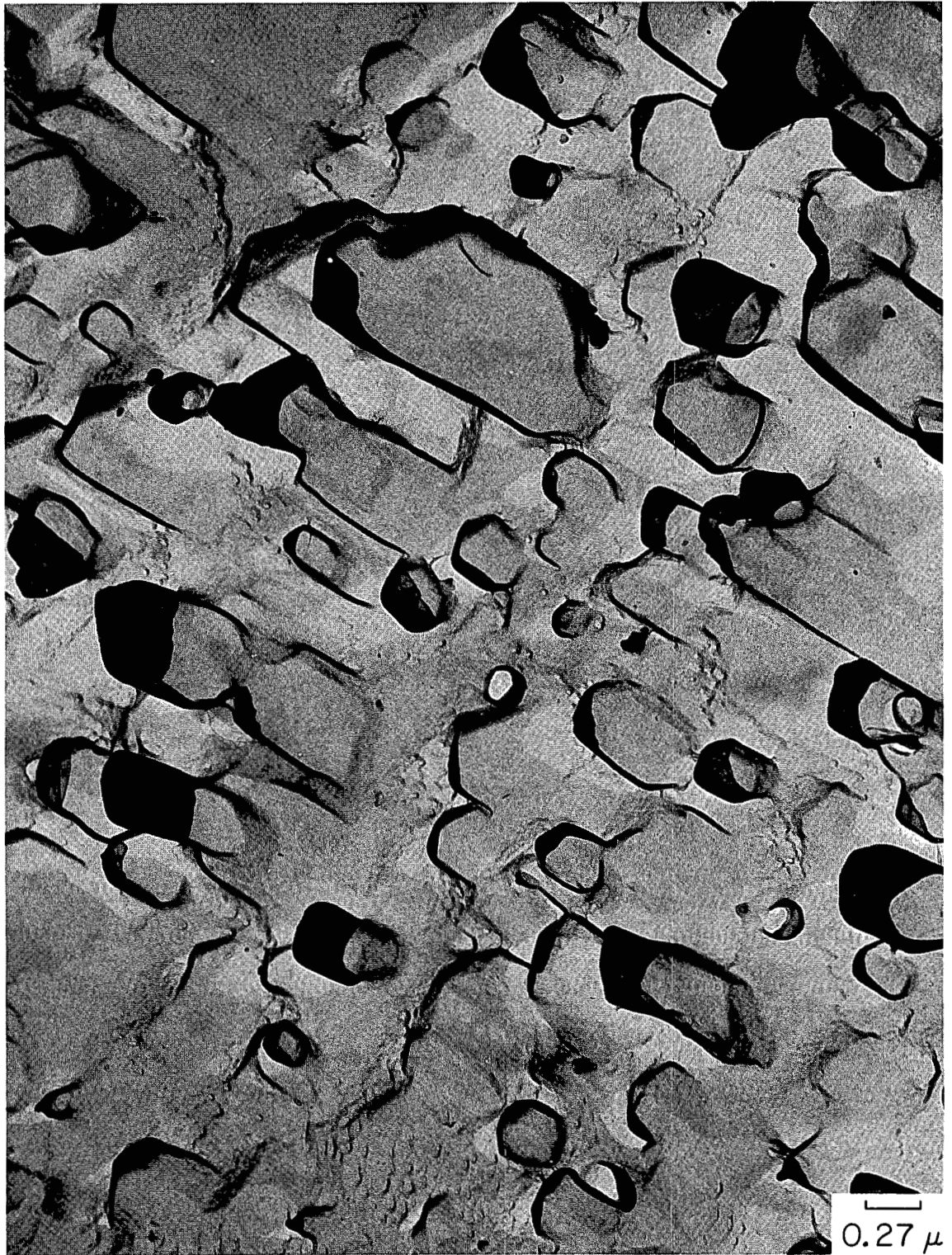
Fig. 21. Polished and Etched Cross Section of \text{Eu}_2\text{O}_3 Microspheres Calcined at 1400-1450°C for 3 hr Showing the Flat Crystal Faces.
