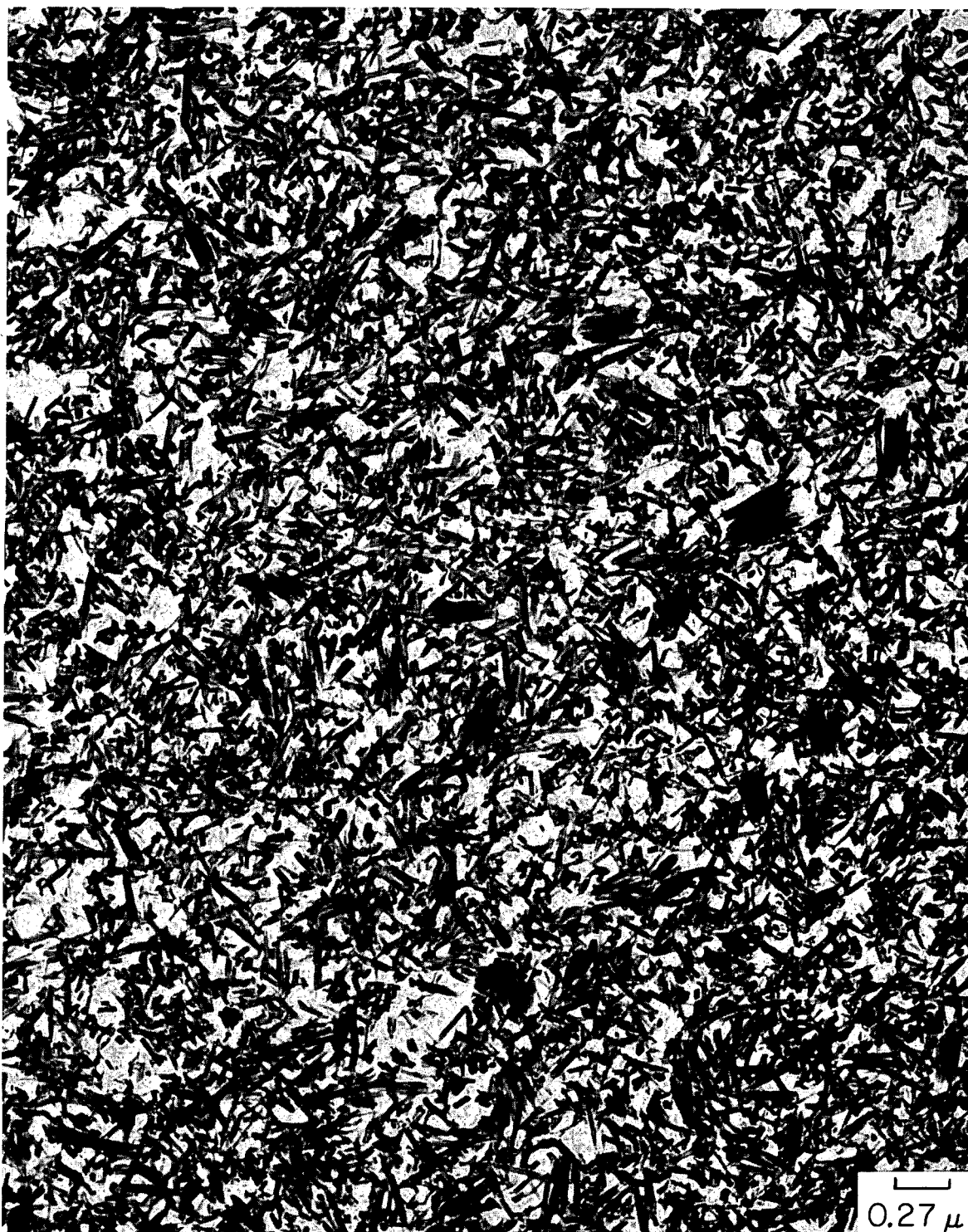
Fig. 23. \text{Eu}(\text{OH})_3 Sol Washed and Aged at 25^\circ\text{C} for 16 hr.
