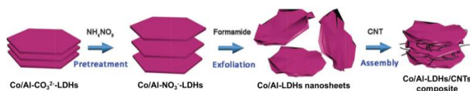
Figure 35. Schematics of each process of assembling the exfoliated Co 2 /Al-LDH/CNT hybrid. 190 Reproduced with permission from reference 190. Copyright 2014 The Royal Society of Chemistry.
