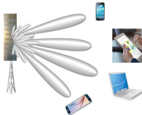
Fig. 1. Simplified illustration of a 5G Massive MIMO system with a base station providing 4 reconfigurable beams to each of 4 users which have LOS but with random AoA and polarization (due to random orientation of terminal).
