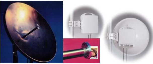
Fig. 2. The original hat feed in ring-focus reflector originally developed for satellite-TV reception at 12 GHz (left). The inserted small picture shows the feed with a matchbox behind it. The innovative use of a corrugated soft-type metasurface is clearly seen. The photos in the background to the right are hat-fed reflectors as used in Ericsson's MINI-LINK for two different reflector sizes.
