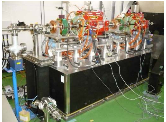
FIG. 4. (Color) View of the final doublet installed on its rigid mechanical support system.
