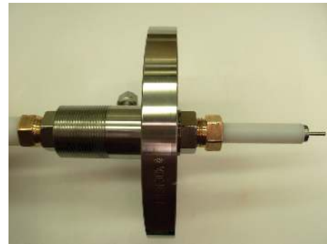
FIGURE 23: The NEXT-DEMO high-voltage feedthrough, designed and built by Texas A&M.
