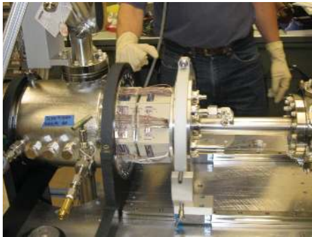
FIGURE 31: The NEXT-DBDM prototype, operating at LBNL. Insertion of the time projection chamber into the stainless-steel pressure vessel.
