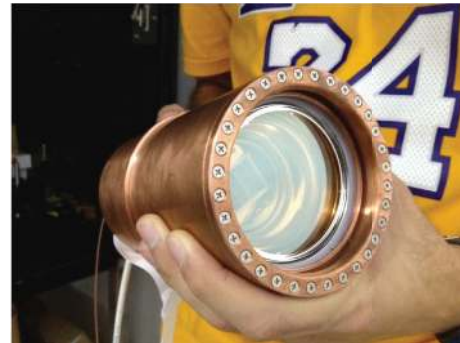
FIGURE 12: The pressure-resistant enclosure or “can” protecting the PMTs inside the pressure vessel.
