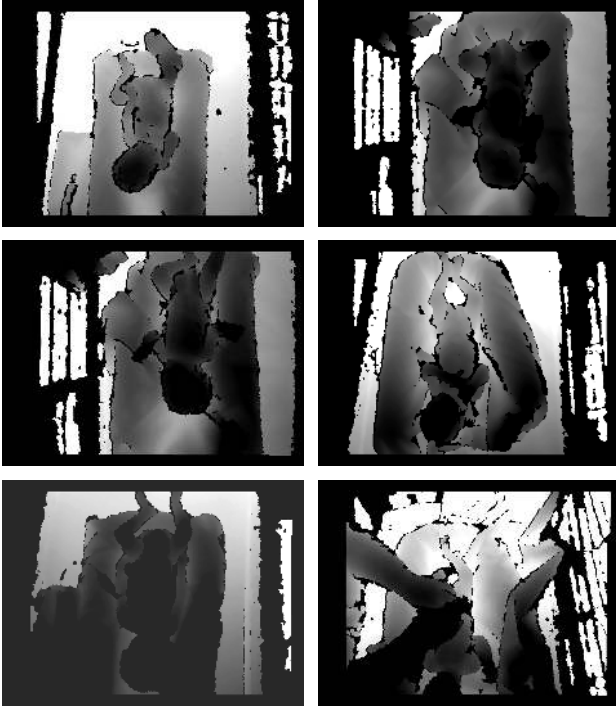
Fig. 6: Challenges in the babyPose dataset, which was acquired in the actual clinical practice, include different poses of the depth sensor with respect to the infant, presence of limb occlusions (both self-occlusion and due to healthcare operators), different number of visible joints in the camera field of view and presence of homogeneous areas with similar or at least continuous depth.
