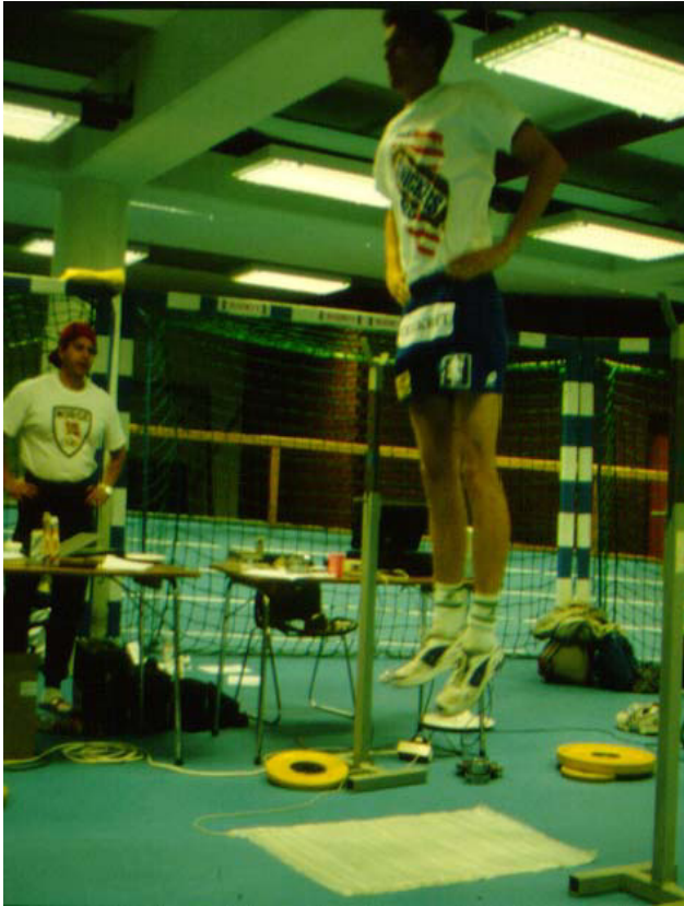
Figure 2. Illustration of the experimental setup for the jump tests. During all tests the players jumped on a contact mat connected to a computer, making it possible to compute jumping height (Bosco et al. 1983).
