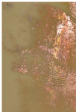
Fig. 10 Etched fingerprint remaining on PCB
