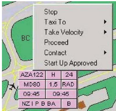
FIGURE 7. The set of possible commands available to the ground controller for a departing flight.
