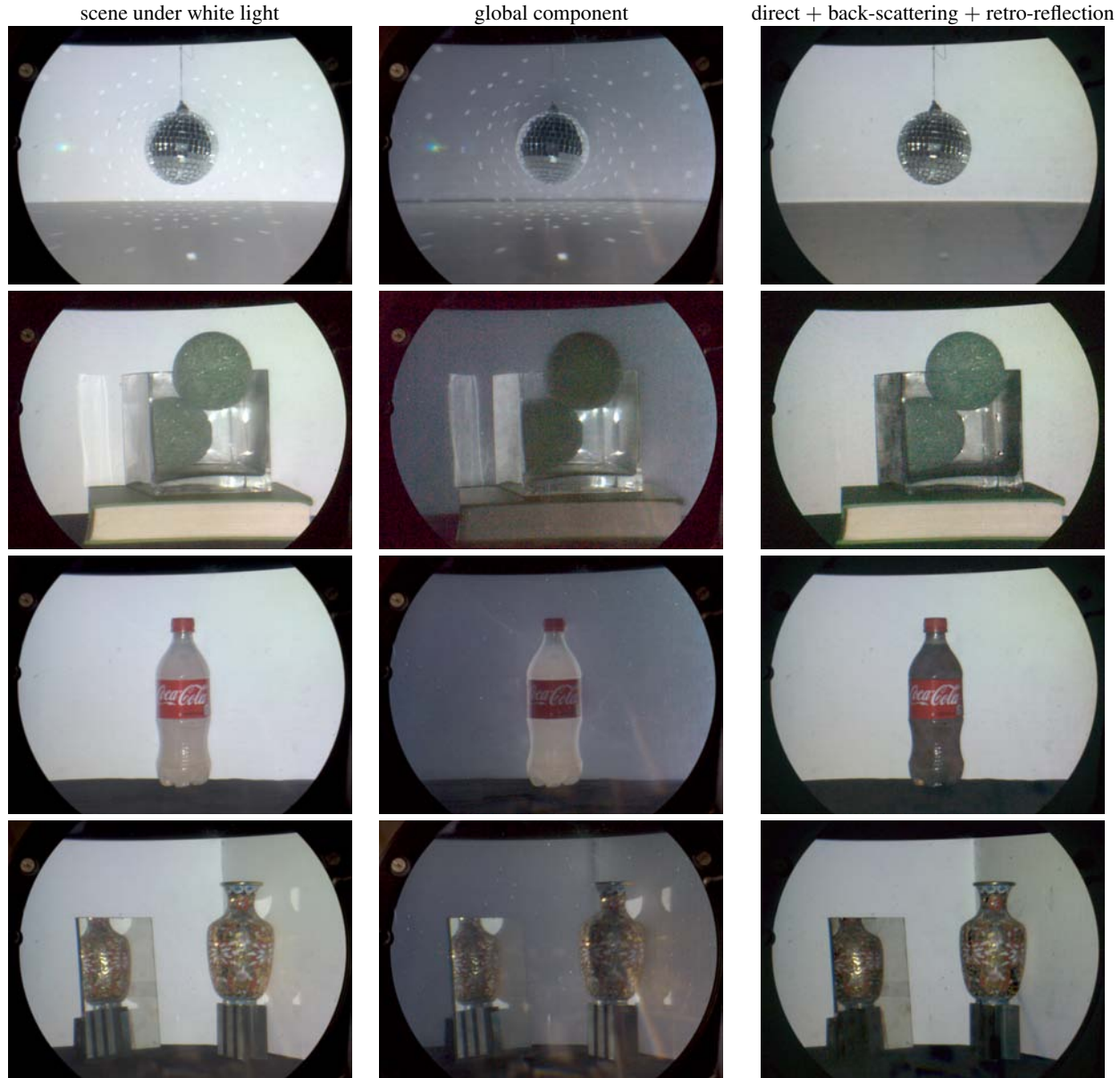
Figure 12: Left to right: Photo of scene under white light, global component of scene captured by a single RAW photo, direct component computed by subtracting the global image from the scene under white light. No processing was done on the photos, other than a resize, flip, white balance, gamma correction and crop. All scenes use 512 primal-dual codes, with the exception of Row 4 which uses 1024 codes. Row 1: A disco ball produces high frequency light transport across the scene, with diffuse inter-reflections occurring near the edge of the floor. Primal-dual coding cleanly separates the photo into its direct component and its global component, which contains inter-reflections and specularities. Row 2: A scene composed of two styrofoam balls inside a glass container generates specular reflections, sub-surface scattering and caustics. We used small aperture to photograph this scene in order to avoid pixel saturation due to caustics. The photo is slightly noisier as a result. Row 3: A coke bottle filled with milky water strongly scatters light that enters the bottle. Row 4: Observe that the direct component contains none of the light that is reflected by the mirror (left) onto the vase (right) and the wall. However, the mirror does not appear black in the direct photo even though it has little to no direct component. This is because of back-scattering and retro-reflection (Figure 4c): light leaves a projector pixel, hits the mirror at a point, diffusely reflects off the wall, then hits the mirror at the same point, and returns to the same pixel. This light path will always contribute to the diagonal of the transport matrix and cannot be distinguished from direct illumination using methods that rely purely on intensity, and without regard to arrival time or polarization. Note that according to Equation 7, the variance of stochastic diagonal estimation may be higher for indirect specular transport than for diffuse transport. To compensate for this, we used 1024 primal-dual codes for this scene.
