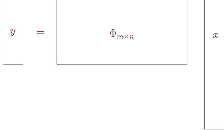
Figure 1: Compressed Sensing model: Matrix form of under-determined system of linear equations. Here \Phi is an m \times n measurement matrix, x is an n dimensional and y is an m dimensional vector, where m \ll n .
