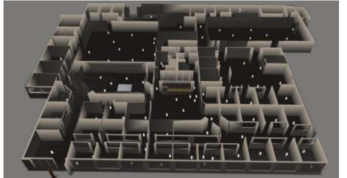
Figure 1. Example problem where 100 simulated robots (white dots) must compute individual collision-free paths in a large, factory-like environment.
