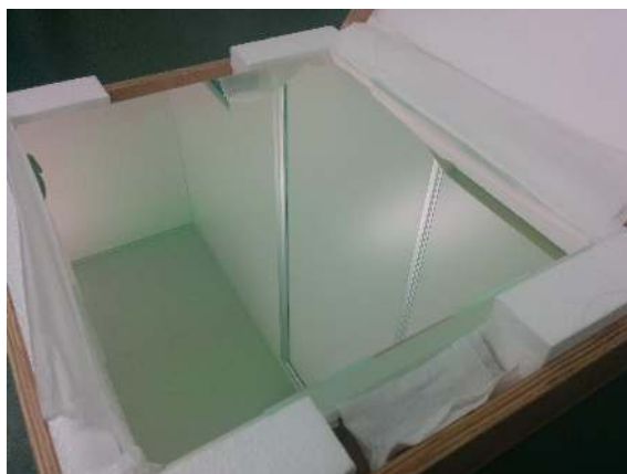
Figure 7. On the left, a photo of the first red dichroic mirror is shown. On the right, the measured reflectance (transmittance) is plotted as a function of wavelength by a blue (red) curve, respectively. The substrate was coated by Asahi Spectra Co., Ltd..
