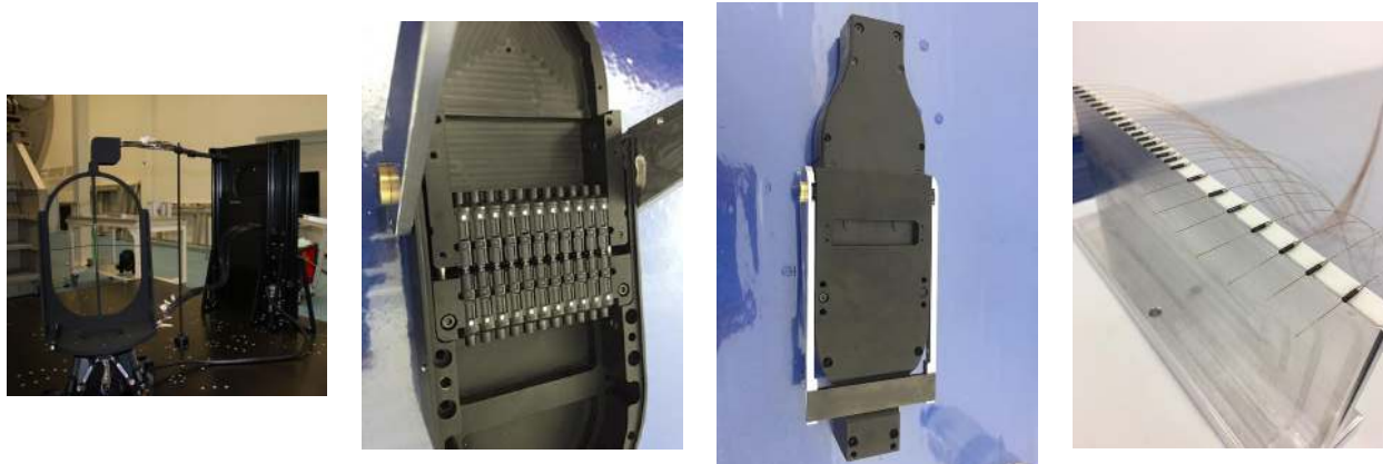
Figure 8. Photos of the parts and assemblies related to the fiber system: 24 (Left) The SpS-side fiber cable system, (middle-left) the inside of the large-format custom-made fiber connector assembly (“Tower connector”) to be installed on the telescope spider structure, (middle-right) the “Tower connector” when mated, and (right) the fibers and ferrules for the PFI-side fiber system in the integration process.
