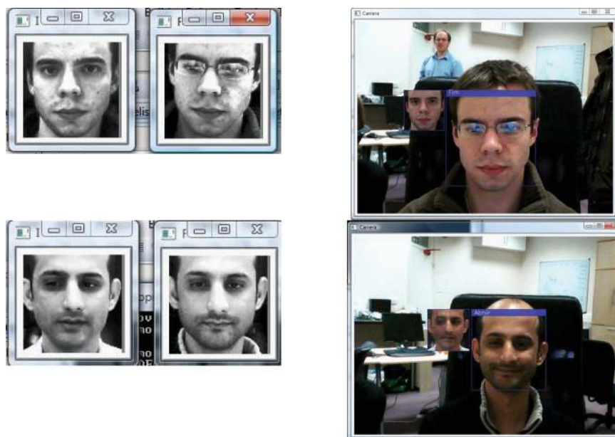
Figure 7. Eigenfaces used to perform real-time recognition using a standard web-cam. Left: Gallery and live pair. Right: Screen shot of system in operation.
