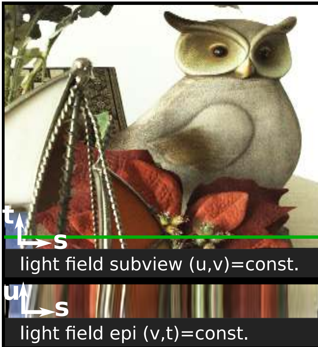
Fig. 7. Light field subview and epipolar plane image (EPI) corresponding to the green line in the subview. The images represent different slices of the four-dimensional light field function l(u, v, s, t) . Note the linear structures of constant color in the EPI. These structures correspond to surface points. Their slope is related to the depth of the scene point.
