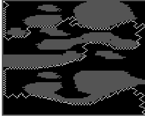
FIGURE H.8. White cells denote the path that was determined with depth-first search.
