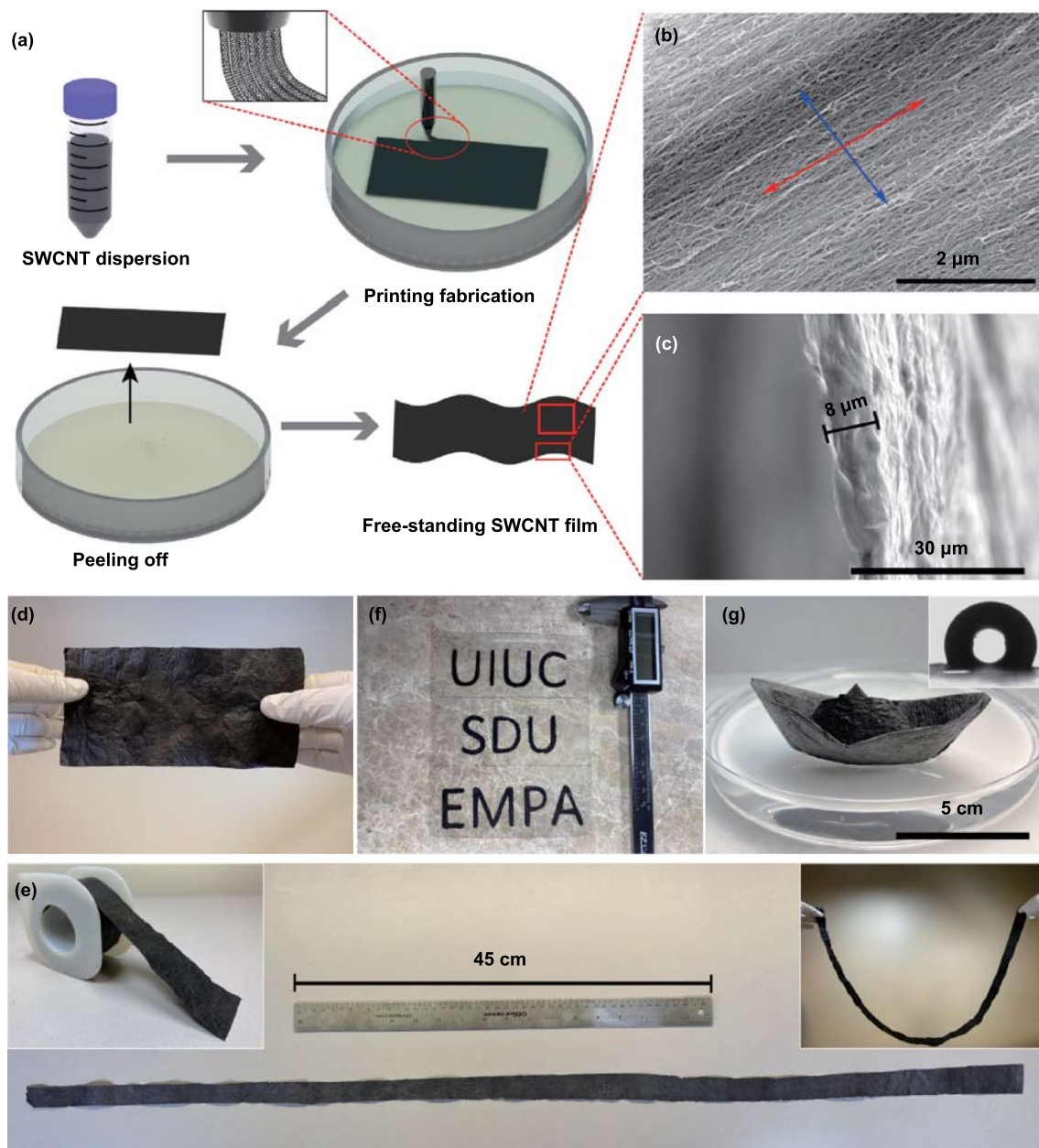
Fig. 1 a Schematic for printing fabrication process of freestanding SWCNT film. b In-plane SEM image of the SWCNTs, showing the aligned SWCNTs in print (red arrow) direction. c Side-view SEM image of the SWCNT film, showing a typical thickness of 8 \mu\text{m} . d Photograph of a large-area ( 10 \times 20 \text{ cm}^2 ) freestanding SWCNT film held by hands. e Demonstration of a meter-long freestanding SWCNT film. f Printed letters of SWCNTs on PET. g Origami boat made from SWCNT film floating on water (inset shows the water contact angle of 125^\circ for the film)
