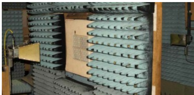
Fig. 3 Measurement setup with 6 \times 6 array of printed squares.
