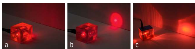
Figure 16: Two identical LEDs are embedded with a 3D printed plano-concave (a) and plano-convex (b) lens. A beam-splitter sends light in two directions (c).
