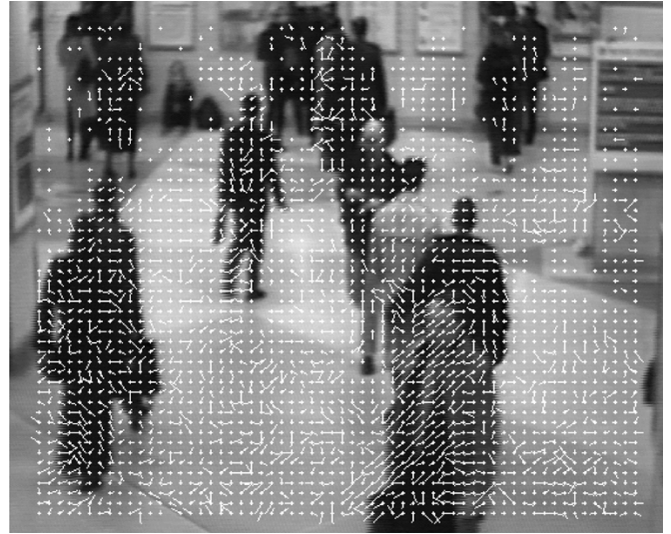
Fig. 2. Typical raw motion vectors (shown in white superimposed on the input image).
