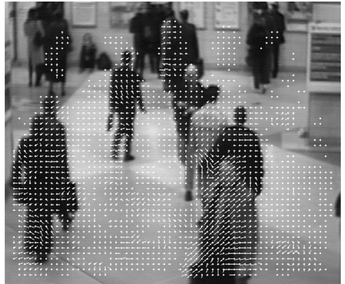
Fig. 3. Typical result after applying mean and median filters.
