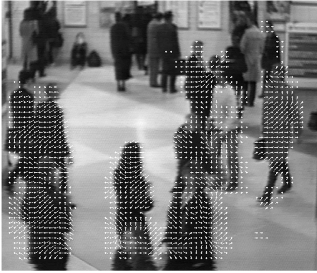
Fig. 5. Extracted motion-vector field after combining it with foreground and interframe conditions.
