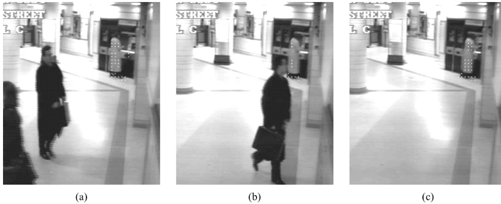
Fig. 16. Dealing with changes in position and pose (images magnified for clarity): (a) Stationary person detected, (b) Person moves to the right, (c) Person redetected after 3 sec.
