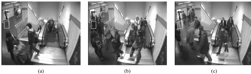
Fig. 17. Maintaining detection of stationary people/objects during occlusion (Rome Metro): (a) Stationary person detected, (b) Detection is maintained during occlusion, (c) Detection is maintained after occlusion.
