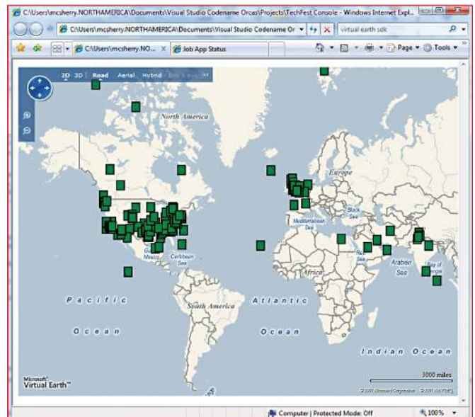
Figure 4. Example output, displaying a representative distribution of the latitude–longitude coordinates of users searching for “cricket.” The computation has differential privacy not because of properties of the output itself, a quite complicated artifact, but because of the manner in which it was produced.
