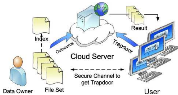
Fig. 1. System architecture of search over encrypted data in cloud computing
