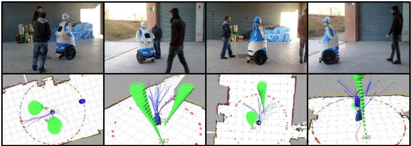
Fig. 7. Examples during experimentation in real environments. Dabo navigates while considering other people on the scene. In the bottom row of the figure appears an interface, where people are plotted as green cylinders and their predictions are drawn in the z axis, which corresponds to time. The tree of paths calculated by the robot appear in blue and the best path is a red line.
