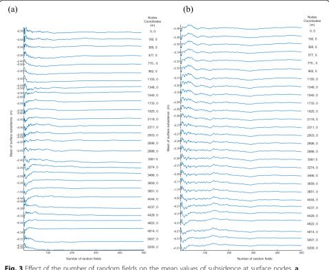
**Fig. 3** Effect of the number of random fields on the mean values of subsidence at surface nodes. **a** Random field of  $E_a$  (case 1,  $I_x = 200$  m,  $I_z = 40$  m). **b** Random field of  $k_a$  (case 2,  $I_x = 200$  m,  $I_z = 40$  m)
