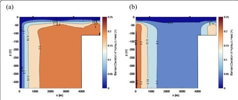
**Fig. 15** Effects of the boundary conditions on the uncertainty of hydraulic head considering the spatial variability of  $k_a$  ( $l_x = 200$  m,  $l_z = 40$  m, COV = 0.8). **a** Hydraulic head boundary condition. **b** Flux boundary condition
