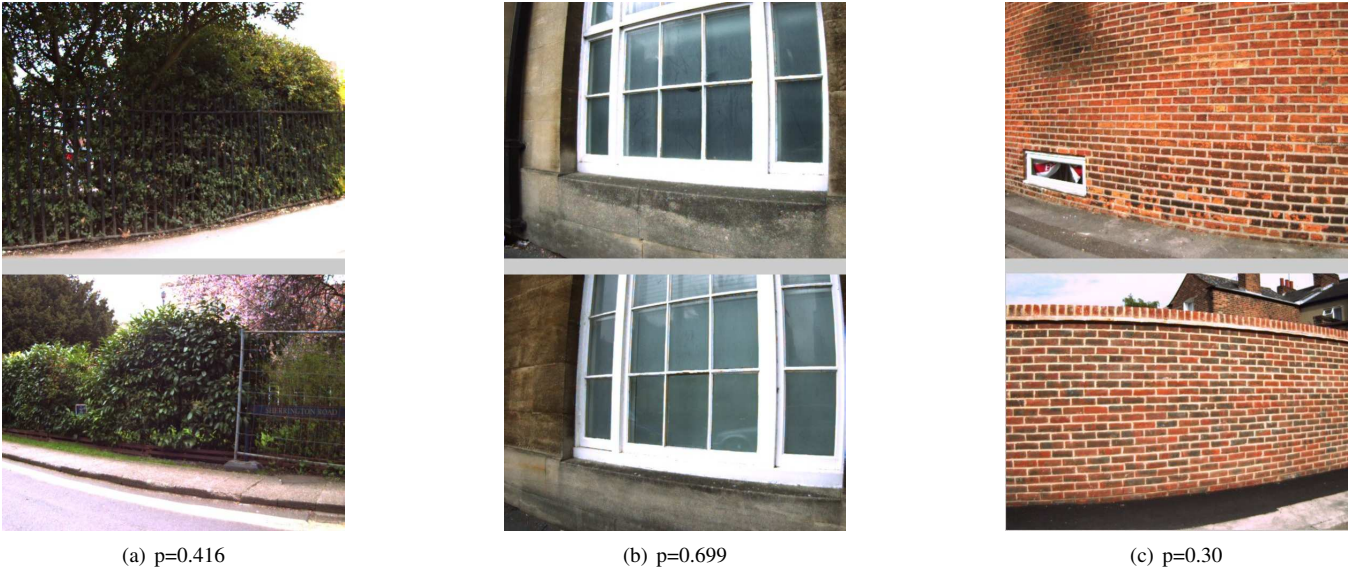
Fig. 3. Some remarkably similar-looking images from different parts of the workspace. The algorithm correctly assigns them low probability of having come from the same place, because our generative model has correctly learned that the words in these images are highly correlated, and hence the images have low distinctiveness. The probability that the two images come from the same place is indicated below the pairs
