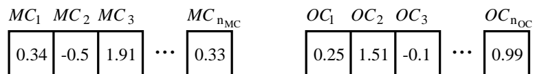
Figure 7.2: Array of n_{MC} and n_{OC} real-valued memory and output cells ( MCs and OCs ) respectively.
