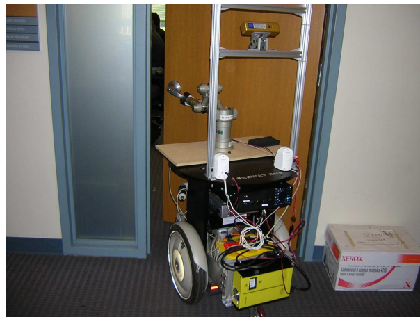
Figure 1: STAIR robot platform manipulating a door during one of our experiments.
