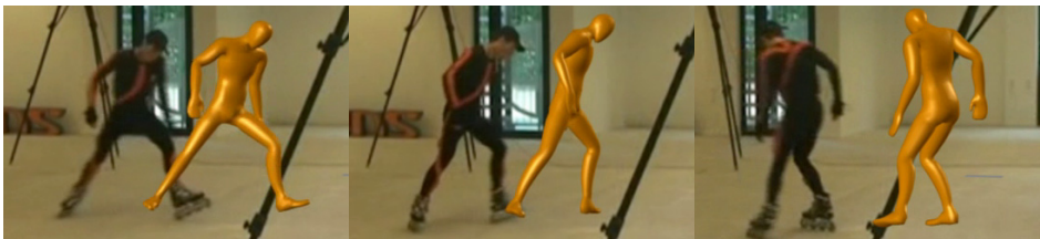
Figure 1.6: Example of inertial motion capture using 17 inertial sensors as well as 3 UWB transmitters on the head and on the feet. The estimated pose is shown in orange. By courtesy of Xsens Technologies.
