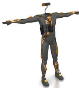
(b) Suit containing 17 IMUs placed on the human body. Courtesy of Xsens Technologies.
