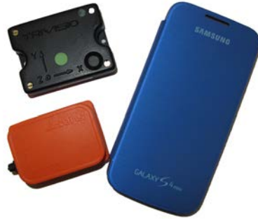
(a) Left bottom: an Xsens MTx IMU (Xsens Technologies B.V., 2016). Left top: a Trivisio Colibri Wireless IMU (Trivisio Prototyping GmbH, 2016). Right: a Samsung Galaxy S4 mini smartphone.
