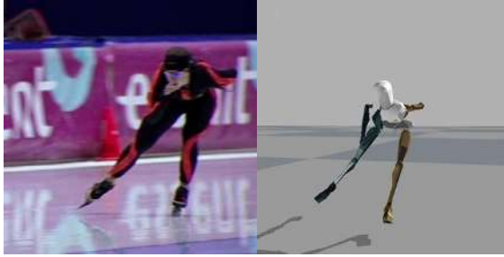
(a) Left: Olympic and world champion speed skating Ireen Wüst wearing sensors on her body. Right: graphical representation of the estimated orientation and position of her body segments.
