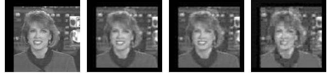
A. Original Image B. Reconstruction from projection of A. MSE = 165.6 C. Reconstruction from sparse coded version of B. MSE = 179.2 D. Reconstruction from quantized version of C. MSE = 295.8.
