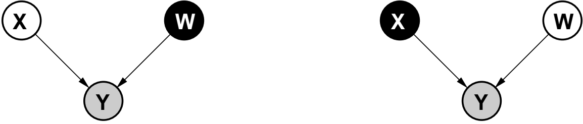
Figure 10: Graphical representation of (a) the standard probabilistic PCA model and (b) its dual representation which also leads to a probabilistic interpretation of PCA. The nodes are shaded to represent different treatments. Black shaded nodes are optimised, white shaded nodes are marginalised and grey shaded nodes are observed variables.
