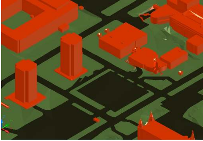
Figure 11: Part of the Université Laval map, chosen for the weighted experiments. Here, different parts of the map have different weights. Buildings are shown in red and have the weight w_{\mathbf{q}} = 0 , ground in represented in green and have the weight w_{\mathbf{q}} = 0.8 , and the streets are shown in black and have the weight w_{\mathbf{q}} = 0.4 .
