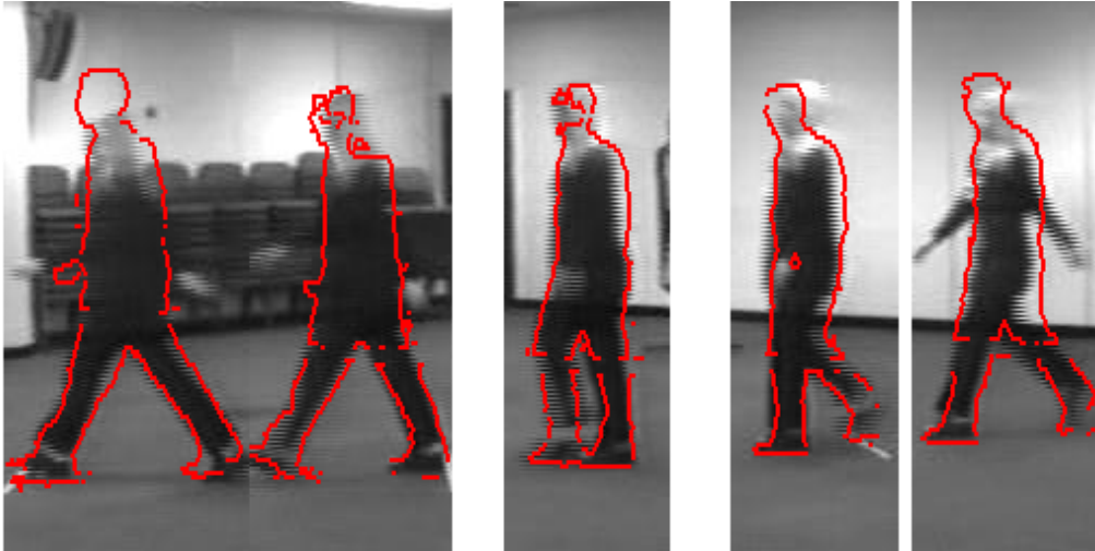
Figure 4. Cropped, sample frames from a tracked sequence. The person tracked does not appear in the training sequences.
