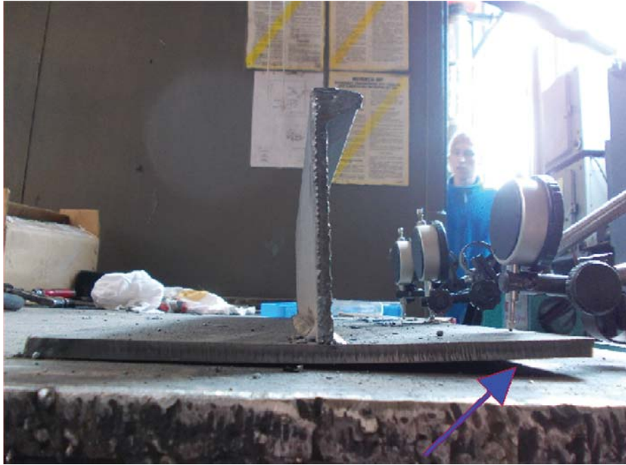
Fig.4. Measurement of angular deformation
