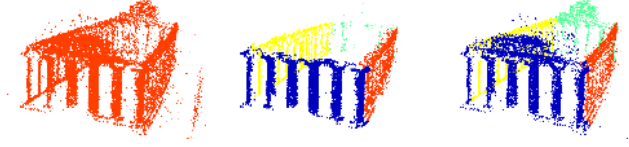
Figure 5. Plane estimation process: The first image shows the entire point cloud, then the planes are estimated in the reduced point cloud and shown in the cleaned complete point cloud.
