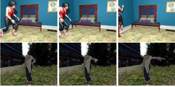
Figure 4: Example generation failure cases. First row: physics violations (passing through a wall). Second row: over-constrained joints and unintended variations.
