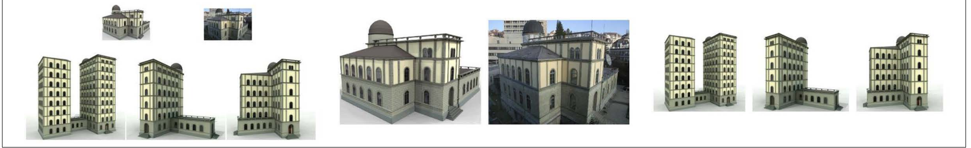
Figure 4 (a) Semper's Sternwarte (Observatory), photograph on the left, rendering on the right. (b) The rule set used to reconstruct Semper's Observatory automatically adapts to any configuration of the underlying mass model. This is a very useful feature to quickly visualize multiple reconstruction-hypotheses of a site.
