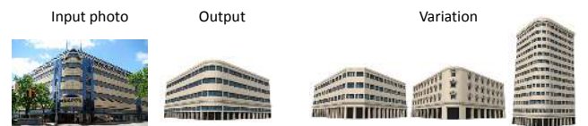
Figure 17: Variation. Our system yields not only a 3D building grammar that is generated based on the input but also a wide variety of 3D geometry by randomly changing parameter values and grammar selections.
