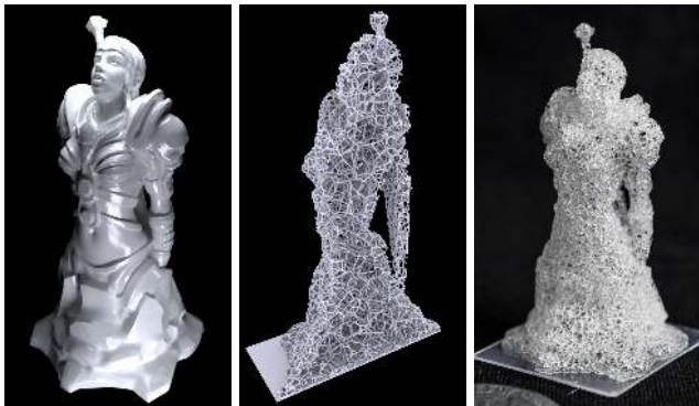
Figure 14: Knight model with a dense crust, and low-density interior. Model: Knight (thing:33804) by andreas.
