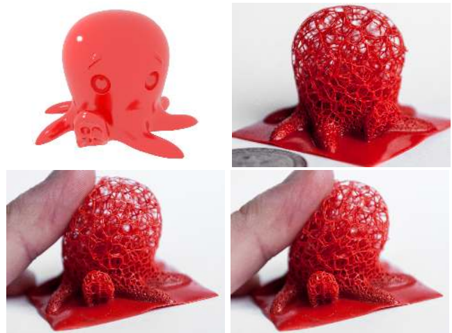
Figure 18: Cute octopus. From left to right: 3D model (original), printed model, printed with deformation (finger pressure). Model: Cute Octopus (thing:27053) by MakerBot.
