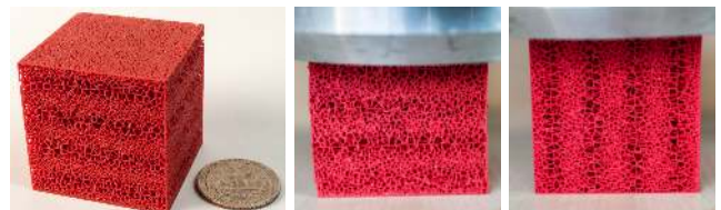
Figure 19: Varying the density in one direction only can also produce parts with anisotropic behavior. The same weight of 8 kg has been applied to the cube placed in different orientations, leading to a visible deformation in the direction of the anisotropy.
