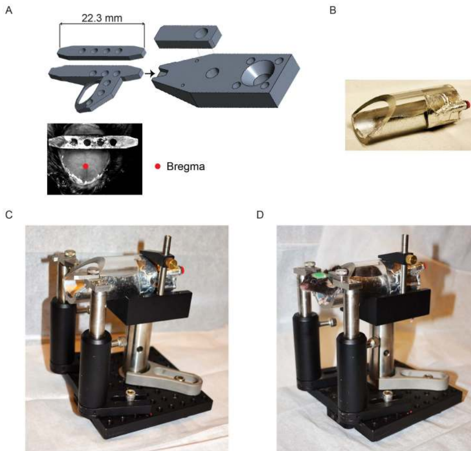
Figure 1. Apparatus for head-fixation. A. Left, two types of titanium head plates. Right, stainless steel head bar holder and clamp (only one of two sides is shown). The head plate is inserted into notches in the holder and fastened with the clamp (right, top) and a thumbscrew (not shown). The simple head bar (left, top) is used when access to large parts of the brain is necessary. The larger head plate (left, middle) provides better stability. The simple head bar was cemented to the skull of the mouse (left, bottom). The head of the mouse (top view) was pointing downward. The skull was outfitted with a clear skull cap [7]. The head bar was aligned at the lambda sutures. The red dot indicates the location of bregma. B. Plexiglass body tube used for head-fixed mice. Mice rest their front paws on the front ledge. The bottom of the tube is coated with aluminum foil to produce electrical contact for electric lickports. The aluminum foil is connected to the red banana socket which will be connected to electric lickports for detecting licking events. C. Example caddy used in training apparatus, assembled from standard optomechanical components (Thorlabs). The head bar holder is mounted towards the left. D. A head-fixed mouse in the caddy. doi:10.1371/journal.pone.0088678.g001
