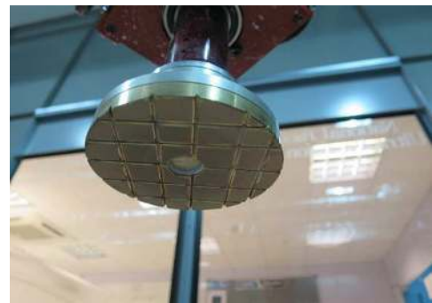
Fig. 3 100mm dia. brass grolishing tool
