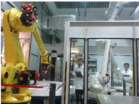
Fig. 2 OpTIC Robot Lab:- 3.05m reach FANUC (near) and 2.55m reach ABB (far)
