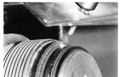
6 Repair of corroded surface by laser cladding (experimental setup)
