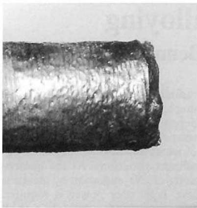
1 Serious workpiece distortion resulting from excessive melting at boundary during laser surface treatment
