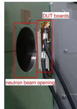
FIGURE 8. Spallation neutron irradiation setup.
