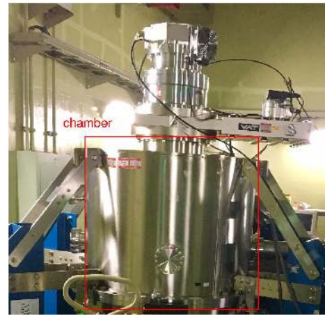
FIGURE 7. Heavy-ion irradiation setup.
