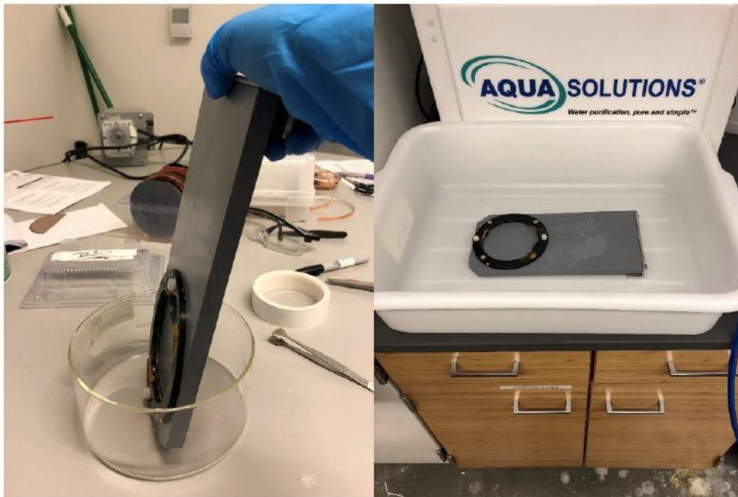
Figure 8. Desirable methods to transfer wafer jig from fume hood to sink after electroplating. Either using a glass beaker (left) or a plastic tray (right).
