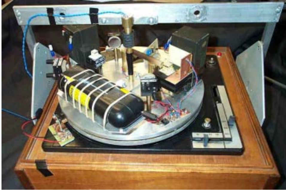
Figure 31: The Flinders experiment. The He-Ne laser is in the lower left hand corner. The glass rod is orientated from upper left to lower right. Rotations are achieved by means of the record turntable. The two rectangular black boxes are batteries.
