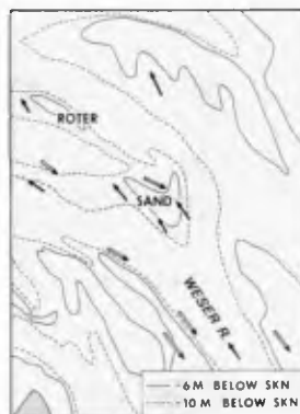
Fig. 17. Bathymetry of the area enclosed by frame in figure 16. Arrows refer to hydrographic data obtained by Barthel (1976). Open arrows indicate flood dominance, solid arrows show ebb dominance.
