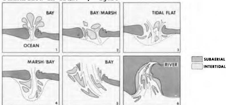
Fig. 10. Tidal inlet morphological models. Frames 1 through 6 reflect an increasing role of tidal currents in inlet sediment dispersal.
