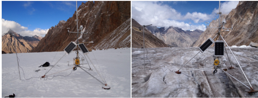
Figure 3. Photographs of AWS1 on Chhota Shigri Glacier taken on 9 October 2012 (left panel) and on 22 August 2013 (right panel) (copyright, Mohd. Farooq Azam). SR50A mounted on a separate pole drilled into the ice, is visible to the left of AWS1.
