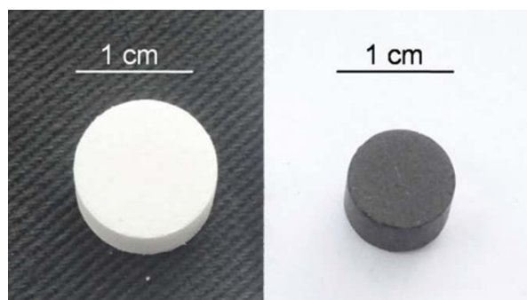
Fig. 7 Photographs of cold compacted SiOC samples before and after pyrolysis.
