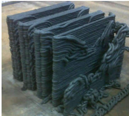
Fig. 3. Testing of buildability of concrete [12]
