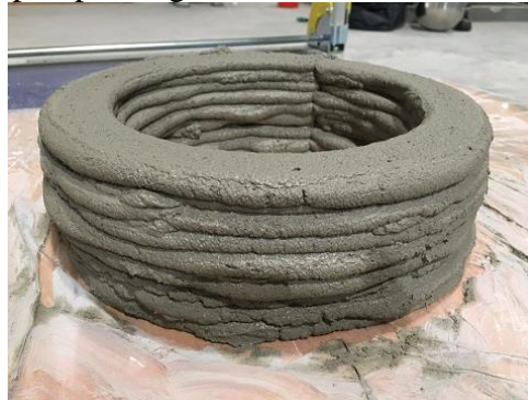
Fig. 2. Experimentation of printing concrete using mix design 6
