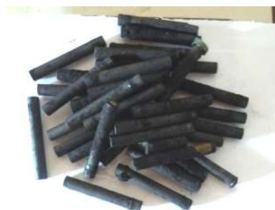
Fig. 2. Carbon rod obtained from used zinc-carbon batteries.
