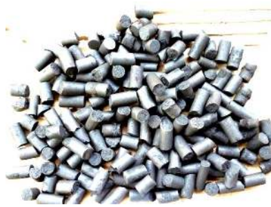
Fig. 3. Carbon rod was crushed in to about 1 cm long.
